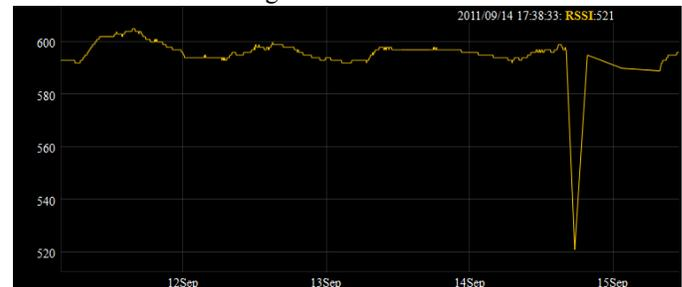
Fig. 6. Significant drop of RSSI caused probably by beam interruption by a bird.
