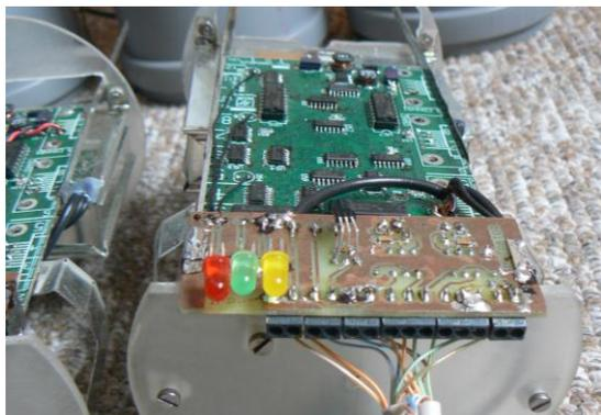
Fig. 2. The realization of TX module. The main processor of the diagnostic module is a microcontroller Microchip PIC18F67j60, which has an integrated physical layer for Ethernet, and does not need many peripherals for their functionality. The microcontroller is connected to 3 temperature sensors DS18B20 placed in the transmitting and receiving tube and also outside to monitor the air temperature. The sensors communicate using 1-Wire protocol. The output of one channel of AD converter is
