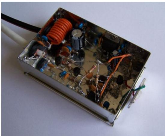
Fig. 2. Design of transmitter part of visible light communication prototype.
