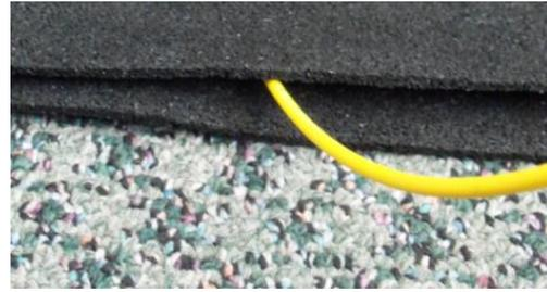
Fig. 3. Illustration of fiber sandwiched between two rubber sheets
