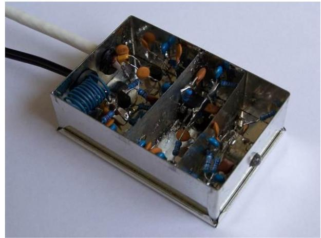
Fig. 3. Design of receiver part of visible light communication prototype.
